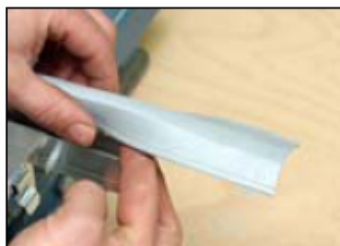
Carefully push seal profile into grooves of internal section by squeezing and replace into housing
