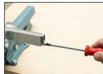
Screw round plastic actuator back onto thread
