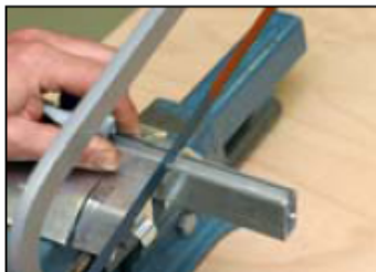
Cut both internal and external aluminium sections after clamping in vice (do not over-tighten) * 708mm cannot be reduced
