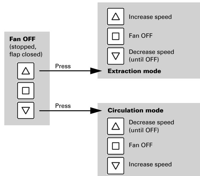
Each time the **OFF** state is reached, the speed variation stops automatically, so that a direct change between extraction and circulation modes is impossible.
